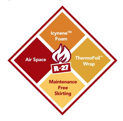
Icynene<sup>TM</sup> foam, Thermofoil, skirting and air space are referred to as the "ThermoQuad". Add in the fifth component, the heat from the pumps, and you actually have a thermo "quinhedron." The important thing to remember is: take any of these five things away, and you will not have proper insulation.
